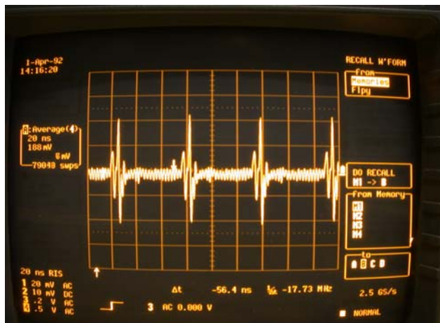
Figure 4: 750 keV chopped beam signal from a gridded pick-up observed on a 1 GHz bandwidth oscilloscope. The central peak of each bunch falls within the RF phase acceptance of the cyclotrons.
