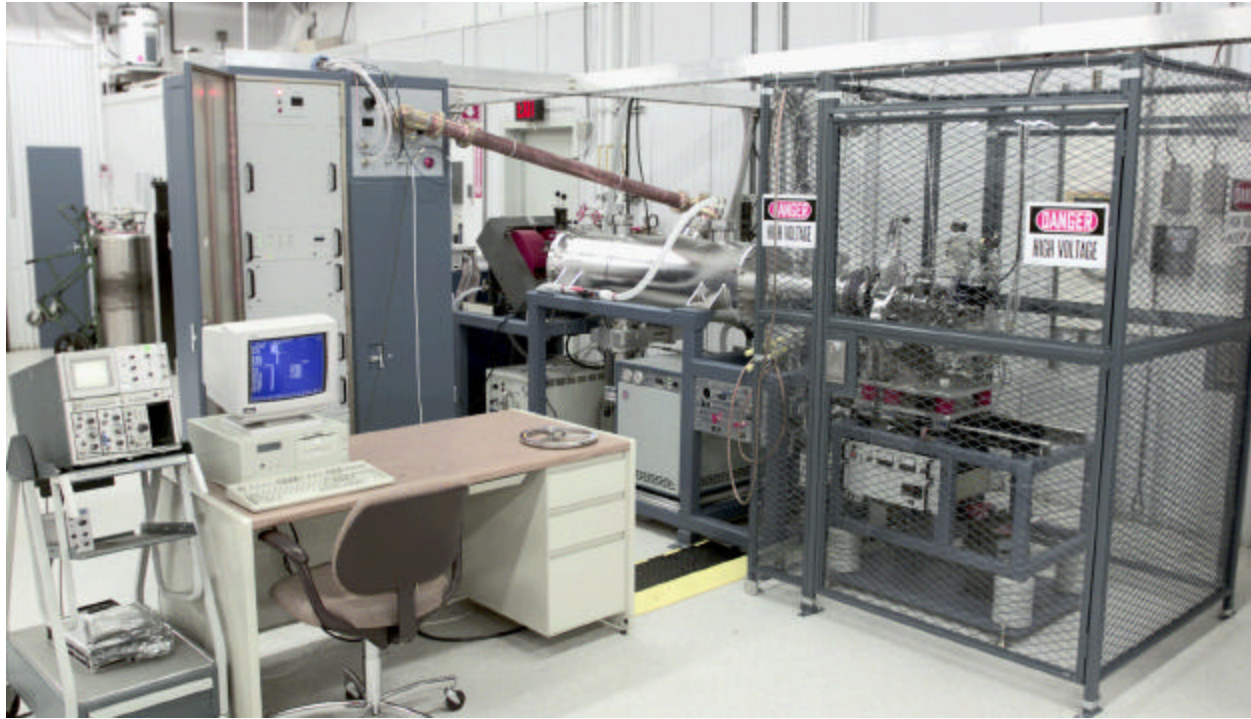
Figure 1. The prototype ^3\text{H} AMS system. The LLNL ion source/sample changer is seen on the right while the AccSys Technology, Inc. RFQ is in the center. The RFQ is 1.38 m long and simultaneously accelerates ^3\text{H} ions to 1.5 MeV and ^1\text{H} ions to 0.5 MeV. Final mass analysis is performed using a small magnetic spectrometer.
